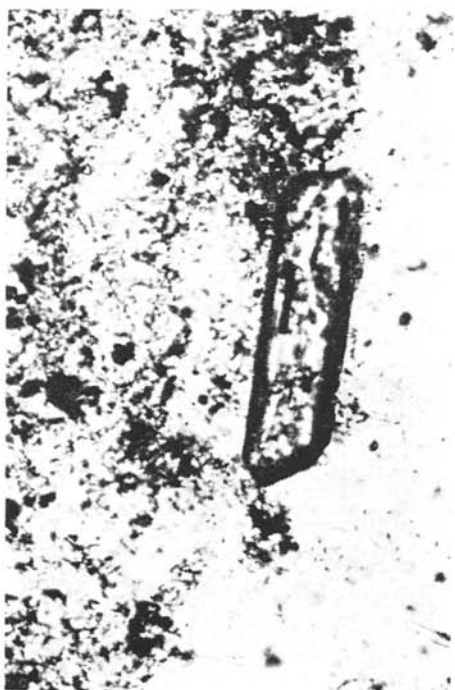
Fig. 5. Columnar monazite crystal enriched in Th, on contact of quartz (right) and sericitized plagioclase (left).
